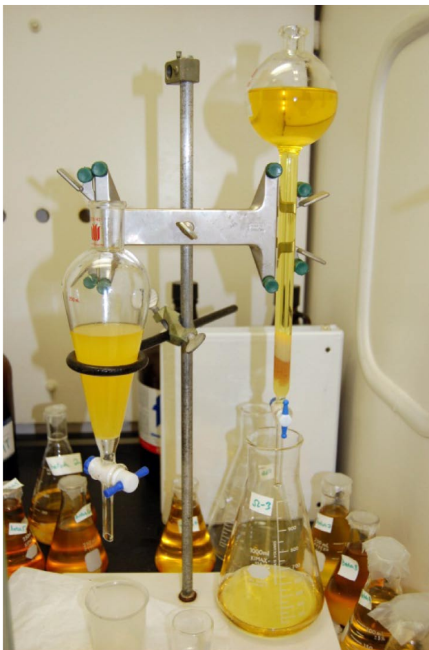
FIGURE 3. ORNL apparatus for washing and polishing biodiesel.
