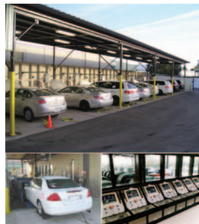
Vehicles on mileage accumulation dynamometers at ETC (top) and SwRI® (bottom) (West)
