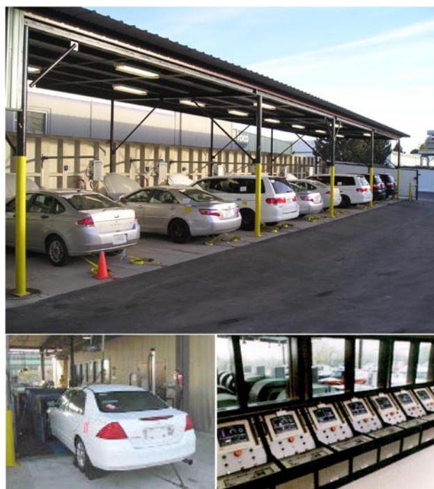
FIGURE 2. Vehicles on mileage accumulation dynamometers at ETC (top) and SwRI® (bottom).
