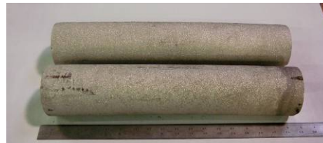
Figure 2: Solid state consolidated billets produced from low cost powder
