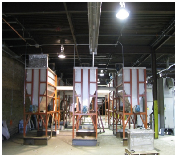
Figure 1: 5000 Pound/hr Flotation Tanks for Recovering Plastics from Shredder Residue
