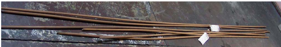
Figure 3: As-hot-rolled bars prior to coiling produced at nearly 100% yield from low cost titanium powder
