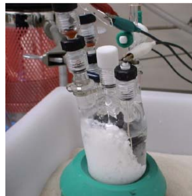
Figure 2: Formation of grams of alane-ligand complex in an electrochemical cell
