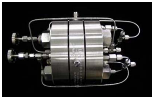
Figure 1: 1.5 lbs/day hydrogen separation test unit
