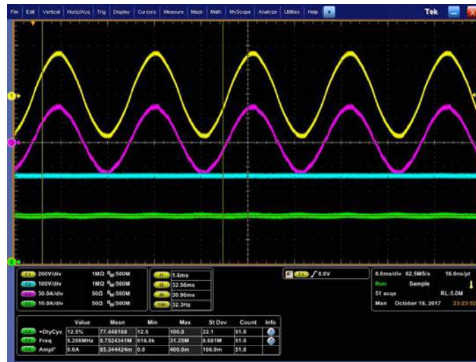
Figure II.1.2 - Level 2 charge waveform, Vout=350Vdc (CH1: Vac, CH2:Vdc, CH3:Iac, CH4:Idc)
