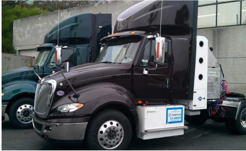
Figure III.9.2 - Transpower Fuel Cell Truck (foreground) and CNG Truck (background)
