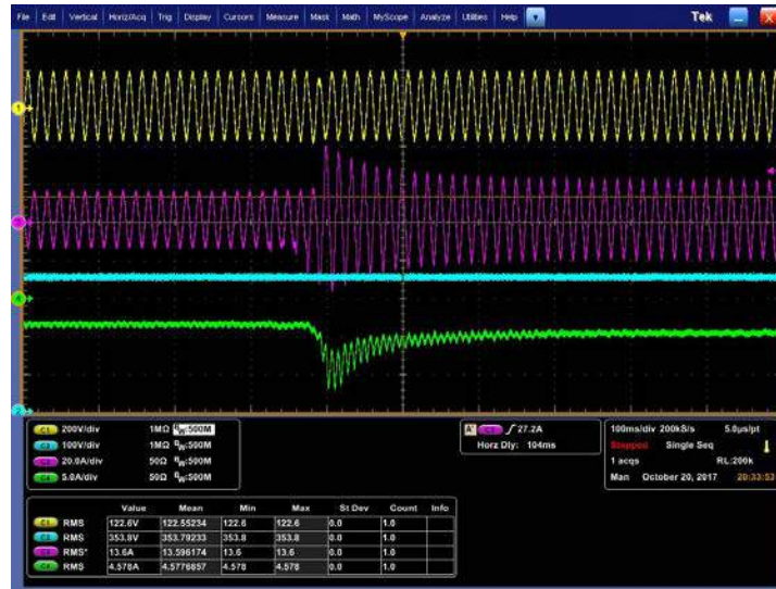
Figure II.1.5 - 120Vac charge waveform, Vdc=350V (CH1: Vac, CH2:Vdc, CH3:Iac, CH4:Idc). Load is 400W incandescent light bulbs + 1266W resistor + 5A drill drilling wood
