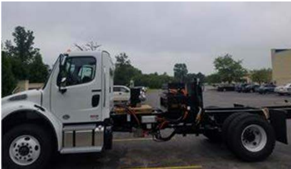
Figure II.8.8 - Hybridized Freightliner M2
