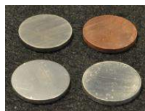
Figure I.14.4 - Cu and invar coupons of 25.4-mm diameter. Photo credits: Douglas DeVoto
