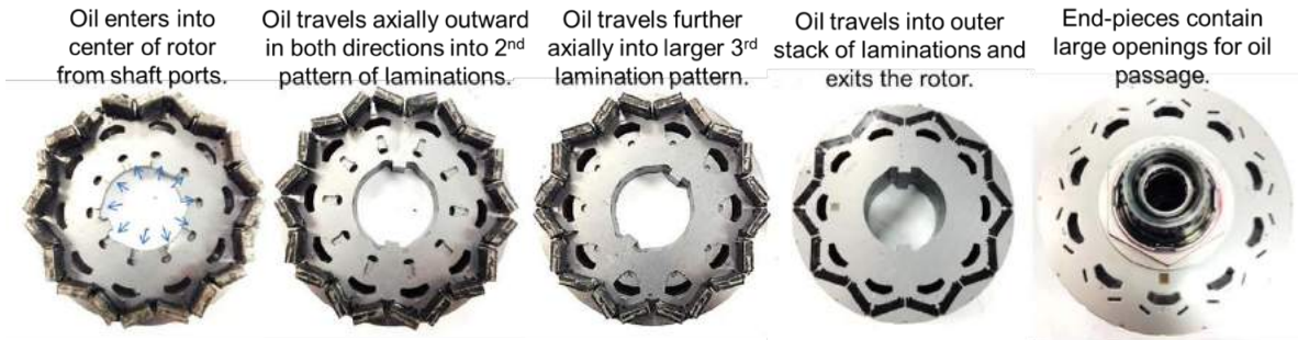
Figure I.7.8 - Oil passageways through several sets of 2017 Prius generator rotor lamination designs.
