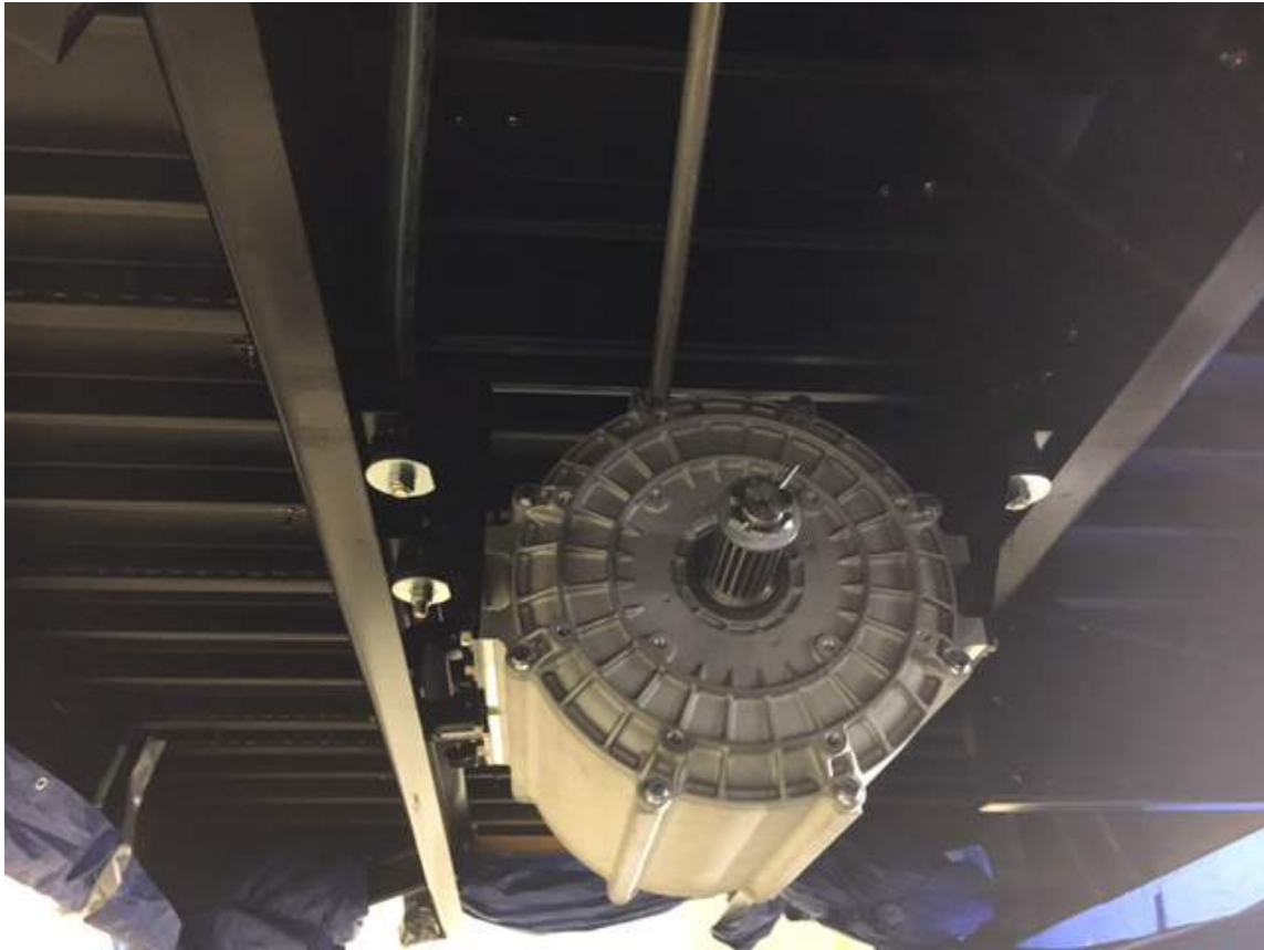
Figure II.5.1 - 3000NM Electric Motor Installed in Bus P1
