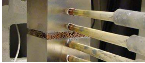
Figure I.15.2 - Sample winding thermal transmission testing Photo Credit: Emily Cousineau, NREL
