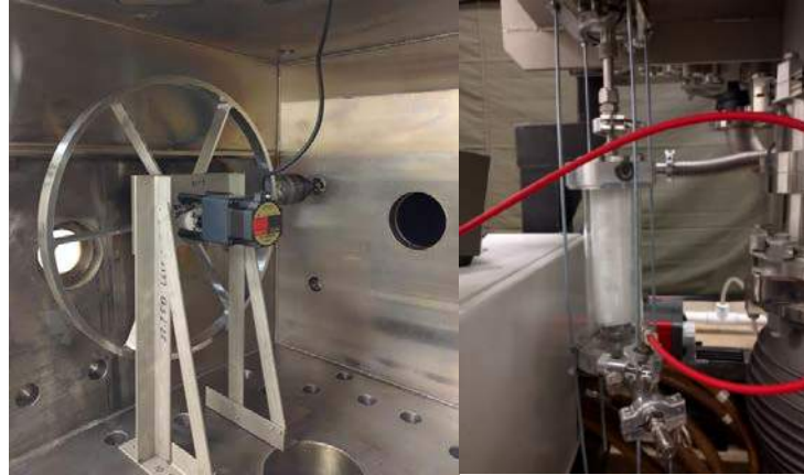
Figure I.12.3 - Rotating-wheel deposition system and the aerosol generator used to make long-length PLZT tapes.
