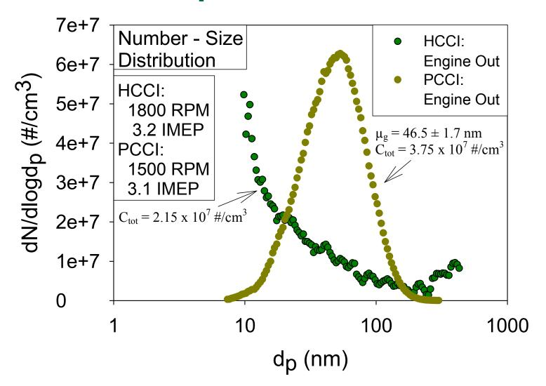
Homogeneous charge compression ignition produced smaller particles
