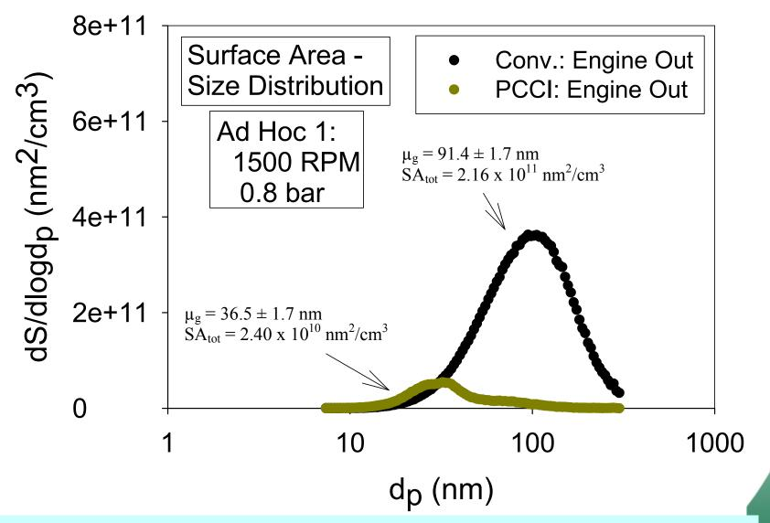
PCCI PM total surface area concentration only 10% of that for conventional mode at Ad Hoc Mode 1
