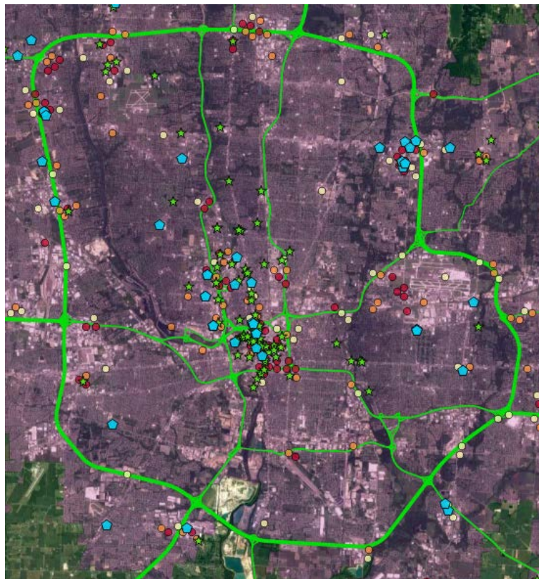
Figure III.4.4 - Simulated PEV charging “hot spots” for L2 public charging (0.3-mi diameter).
