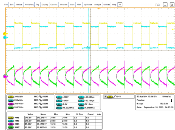
Figure II-37: Single SiC H-bridge test waveforms obtained using the single-phase test bed. The tests were conducted at 250 V, 15 A continuous operation at 20 kHz.
