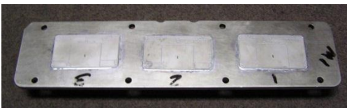
Figure III-151: Substrate to Coolant Manifold Attachment.
