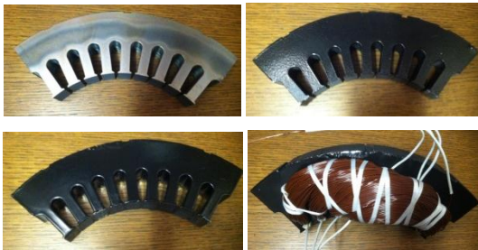
Figure IV-6: Illustration of stator segment. Top: uncoated core sample (left); coated with SolEpoxy 2905-102B (right). Bottom: preheated segment dipped in fluidized DK15-0984 and lap wound with 19 AWG magnet wire (right).
