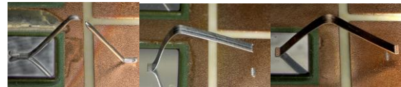
Figure V-55: Failure modes from the left: wire break (left), heel failure from substrate (center), and bond lift-off from substrate (right). (Photo credit: Doug DeVoto, NREL)
