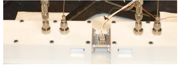
Figure V-94: Heat exchanger installed in test fixture with inlet and outlet temperature and pressure measurements
