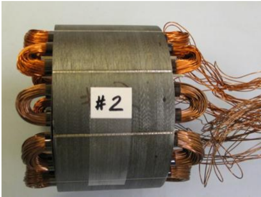
Figure IV-56: Stator constructed with the HT film developed on this project as slot liner.
