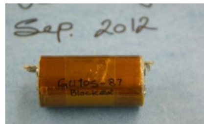
Figure III-155: Blisters on shorted cap.
