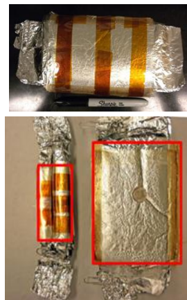
Figure III-133: Stacked capacitor (top) Stacked vs. rolled.
