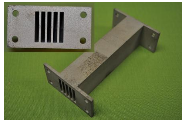
Figure V-33: Baseline aluminum fin block sub-module test section.
