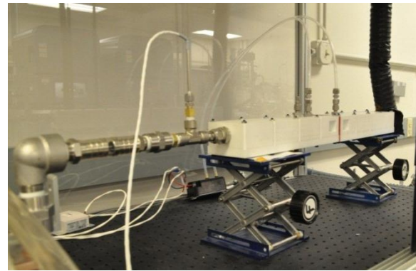
Figure V-32: Test section for testing baseline aluminum fins with two heaters for model validation; pressure calibration testing shown. (Photo Credit: Scot Way, NREL).
