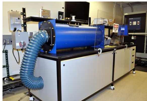
Figure V-15: Photograph (top) and schematic (bottom) of the channel flow experimental setup: (1) compressed air, (2) desiccant dryer, (3) filter/regulator, (4) mass flow controller, (5) laminar flow element, (6) plate heat exchanger, (7) temperature control bath, (8) fin test section, (9) ceramic resistance heaters, and (10) isolation box.
