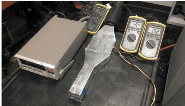
Figure II - 103: Temperature measurement devices and assembled test fixture.
