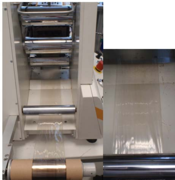
Figure II - 132: Sandia developed high temperature dielectric material extruded at Dr. Collin company.
