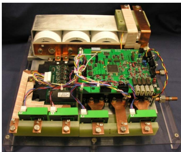
Figure II - 52: An integrated charger prototype using a traction drive comprising a 55 kW motor inverter and a 30 kW generator inverter.
