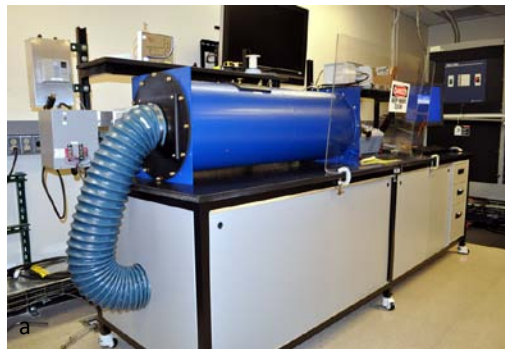
Figure V - 67: System-level air-cooling test bench: a. picture b. schematic.
