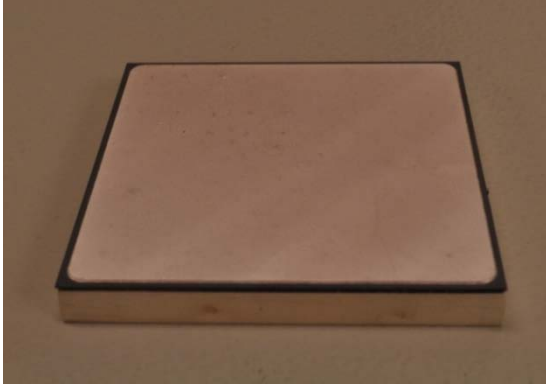
Figure V - 34: Representative metalized substrate/base plate assembly (Photo credit: Doug DeVoto, NREL).
