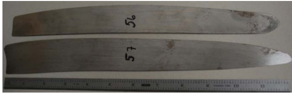
Figure III - 21: Sheets rolled to 14 mil thickness of improved soft magnetic laminates.
