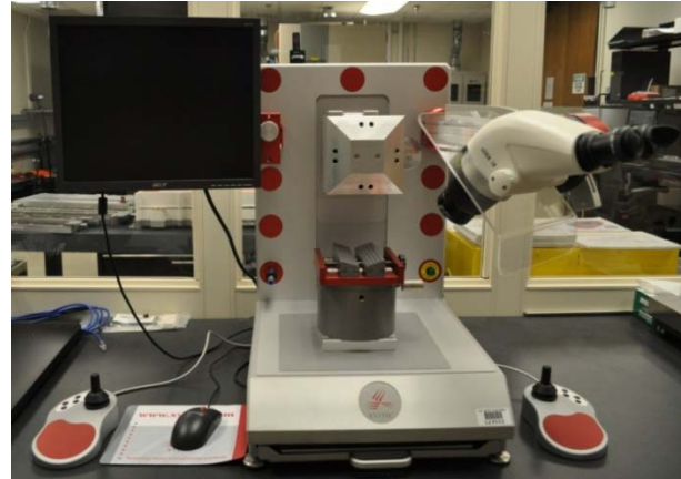
Figure V - 25: Mechanical bond tester (Photo credit: Doug DeVoto, NREL).
