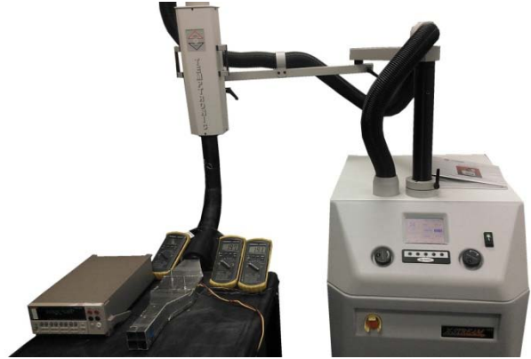
Figure II - 104: General test setup; Tempronic X-stream 4310 air temperature and flow control (on right).
