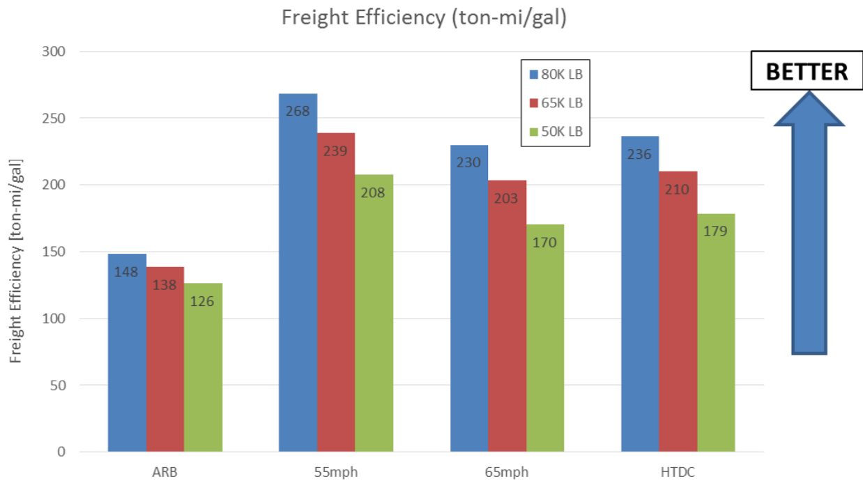
Figure VII.5.4 - Fuel consumption for different cycles and vehicle weight
