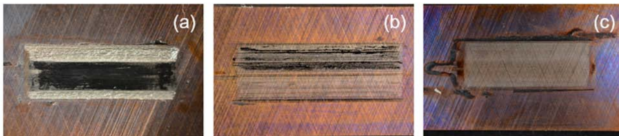
Figure VI.1.1 - Micrographs of gray cast iron liner surfaces subjected to a scuffing load test at flow rates of (a) 0.1 \mu\text{L}/\text{min} , (b) 0.2 \mu\text{L}/\text{min} , and (c) 0.5 \mu\text{L}/\text{min}
