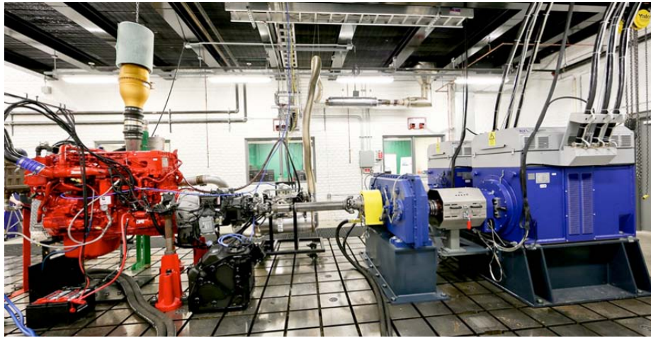
Figure VII.5.1 - ISX450 engine with UltraShift Plus AMT under test in the powertrain test cell at ORNL's VSI Laboratory
