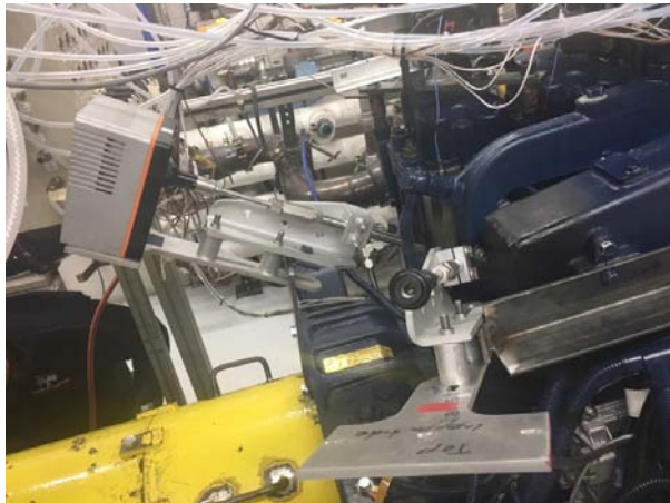
Figure III.3.3 - Camera arrangement for optical in-cylinder measurement. Two optical probes were positioned toward the spark plug for viewing of ignition point and flame propagation. Cylinder #6 (rear cylinder) was used for instrumentation access. Top view. (Figure source: Bosch)
