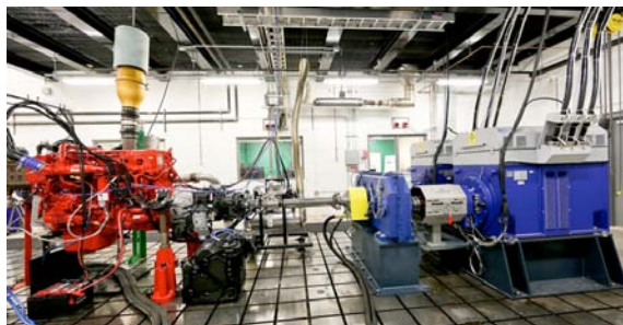
Figure 21 - ISX450 engine with UltraShift Plus automated manual transmission under test in the powertrain test cell at Oak Ridge National Laboratory's Vehicle Systems Integration Laboratory (Deter, report VII.5)
