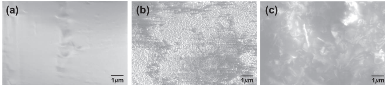
Figure VII.3.6 - SEM images of the (a) unfilled SBR, (b) SBR filled with GnP, and (c) SBR filled with functionalized GnP and SnF
