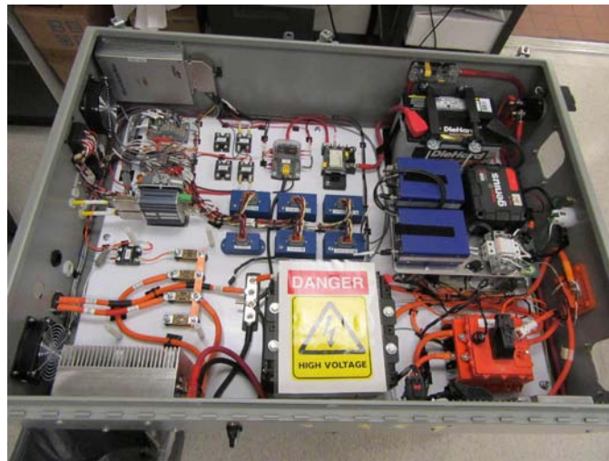
Figure V.9.6 - Control hardware (Source: Eaton)
