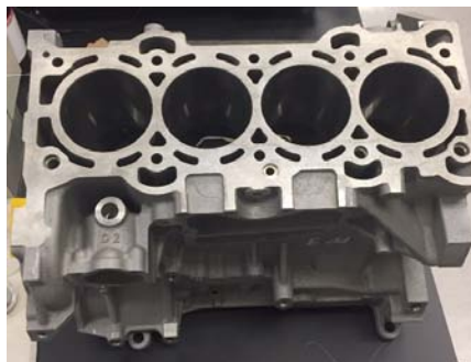
Figure 19 - Plasma transfer wire arc coated cylinder bores in a linerless engine block (Source: Ford Motor Company) (Gangopadhyay, report VI.7)
