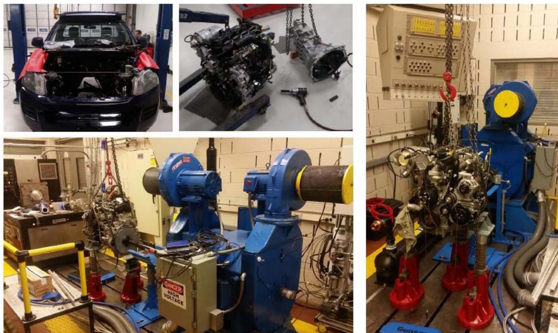
Figure V.9.1 - Isuzu engine unmounted from the vehicle, mounted on the dynamometer (Source: Eaton)
