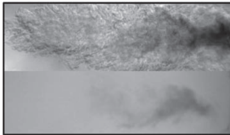
Figure 2 - Example diffused back-illumination extinction imaging images using the original setup (top) and optimized setup (bottom). The light and dark regions in the top image are caused by beam steering and introduce significant error when attempting to quantify soot or liquid penetration in high-pressure sprays (Pickett, report I.3)
