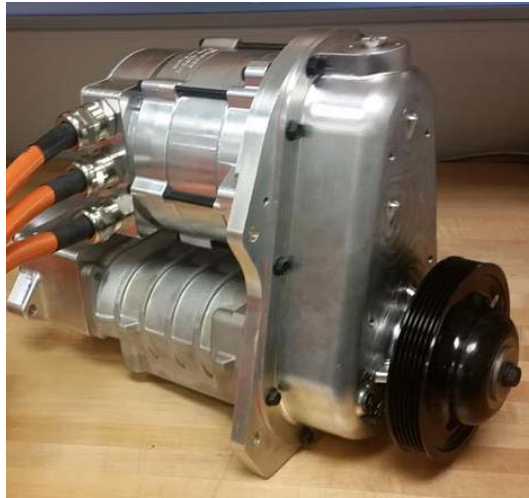
Figure V.9.3 - EAVS unit (Source: Eaton)
