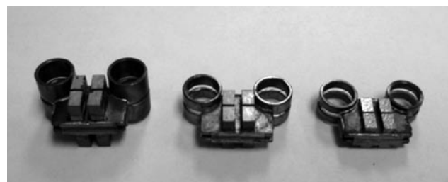
FIGURE 3. From Left to Right, Typical High-, Medium- And Low-Temperature TE Engines
