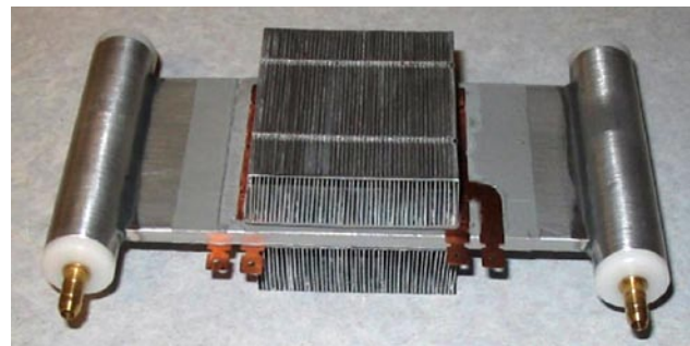
FIGURE 3. Prototype liquid-to-air TE heat pump design used for validation testing of various manufacturing methods.
