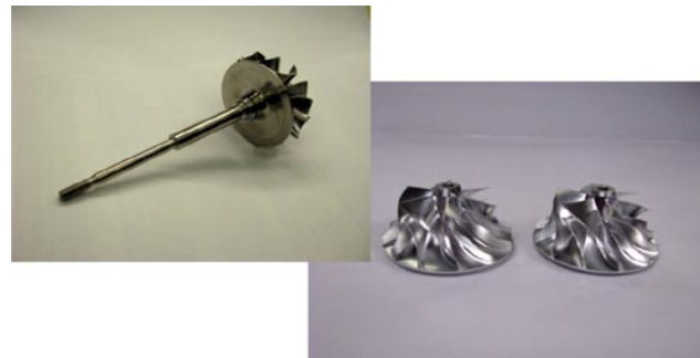
FIGURE 1. Mixed Flow Turbine and Compressor Wheels were Fabricated
