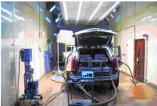
FIGURE 4. Instrumented Mule Vehicle in the Delphi Climatic Wind Tunnel
