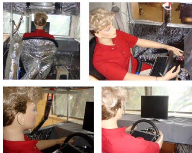
FIGURE 2. Thermal Mannequin Inside the Mock-Up Vehicle in the UCB Environmental Test Chamber
