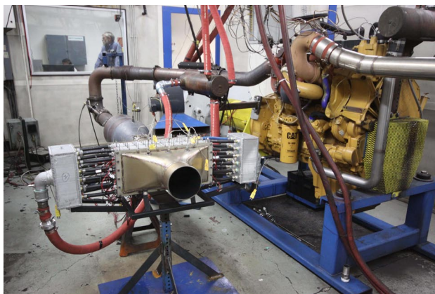
FIGURE 6. 1-kW TEG for a BFV attached to a diesel engine dynamometer.
