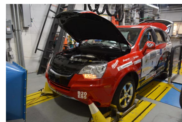
University of Wisconsin Reactivity-Controlled Compression Ignition Hybrid Vehicle on the ORNL Chassis Dynamometer undergoing Drive Cycle Evaluations (Curran, report II.18)
