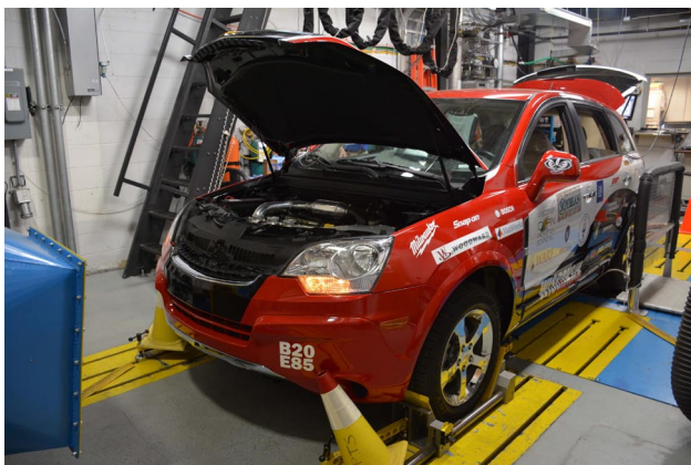
FIGURE 4. University of Wisconsin RCCI Hybrid Vehicle on the ORNL Chassis Dynamometer undergoing Drive Cycle Evaluations
