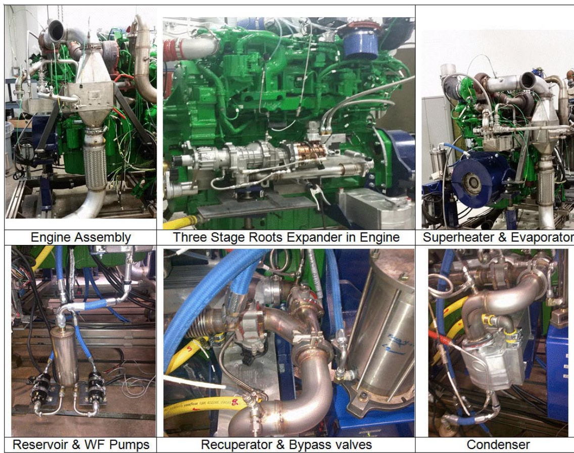
FIGURE 5. Roots ORC System Integrated onto the Engine
