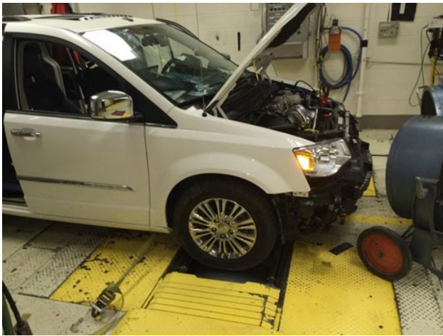
FIGURE 3. Vehicle Installed in Chassis Rolls Emissions Test Cell
