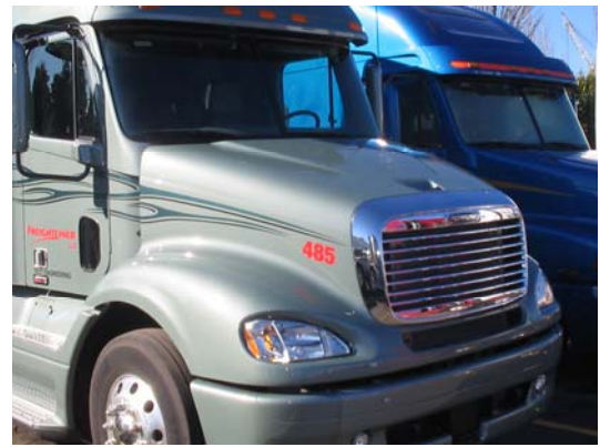
Figure 2. Prototype truck hood for hybrid composite molding.
