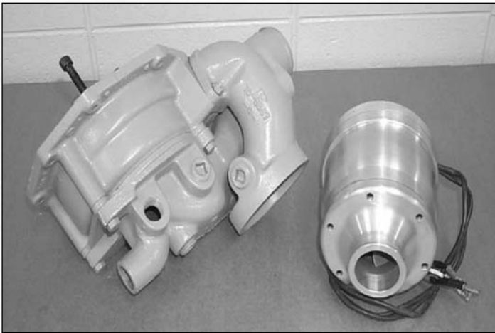
Conventional mechanical water pump (left) and equivalent More Electric electrically driven water pump.
