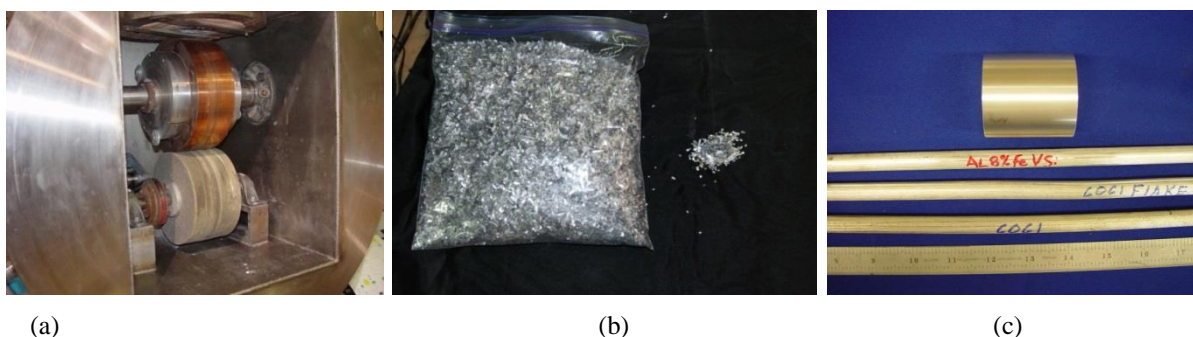
Figure 1. (a) Picture of the PNNL flake melt-spinning machine with the front chamber removed; (b) typical RS flake product produced with the melt-spinning equipment; (c) photograph of the canned RS flake billet (top) and the extruded rod.
