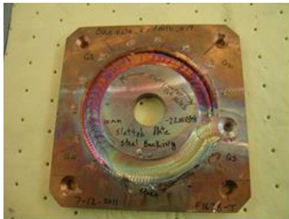
Figure 6. Surface-breaching void defect due to weld parameters that did not deliver enough weld energy for a consolidated joint.
