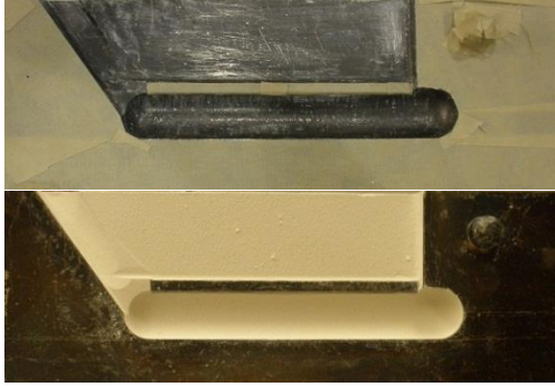
Figure 3. Cast iron mold for casting torpedo sample: (a) without coating and (b) with coating.
