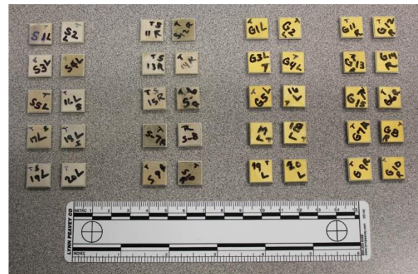
Figure 7. Processed DBC sandwiches ready for shear-strength-testing. The effects of plating (silver versus gold) and printing method (screen versus stencil) on shear strength are under evaluation.
