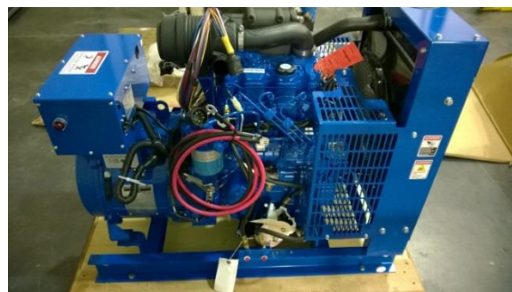
Figure 11. Northern Lights stationary generator.
