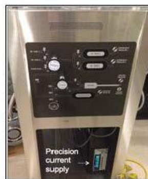
Figure 1. “Alpha” version of Protochips commercial gas manifold for computer-controlled operation of a gas reaction holder for the JEOL 2200PS ACEM.
