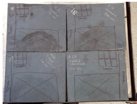
Figure 4. Weld plate cast with modified SAE 15V22 with test sample cut locations marked.
