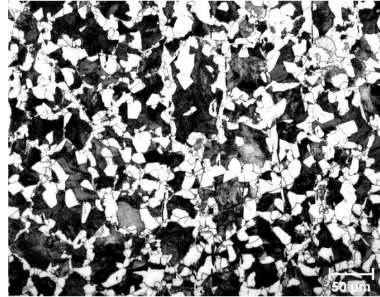
Figure 10. Microstructure of the parent material, 1538-MV micro-alloyed steel. Presence of ferrite and pearlite phases is evident.
