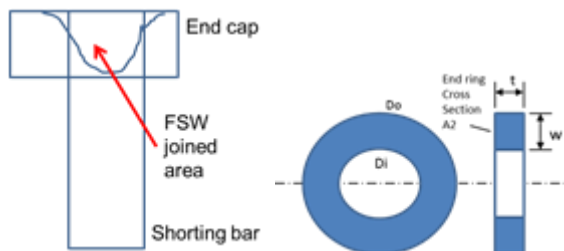
Figure 3. Schematic of the end cap/shorting bar joined area.
