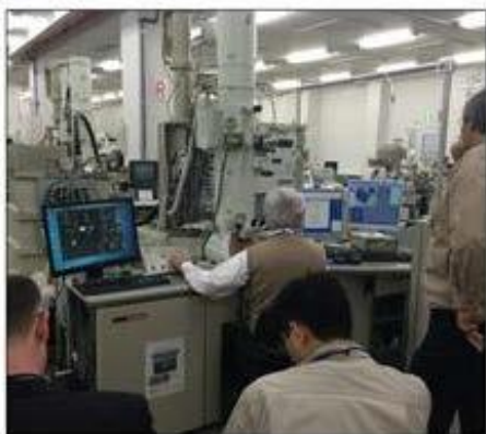
Figure 3. Dr. Larry Allard operating the JEOL 2100 TEM/STEM instrument at the JEOL factory during the qualification test/test out of the Protochips alpha-version commercial gas reactor system.
