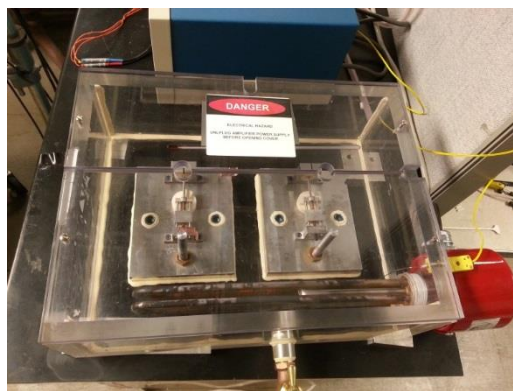
Figure 1. An immersion heater (MTO-110/120 E1) is installed in the tank of piezodilatometer that can heat the electronic liquid to a target temperature.
