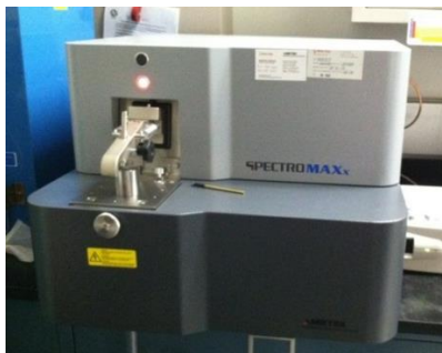
Figure 1. In-house SPECTROMAXx spark optical emission spectroscopy metal analyzer.
