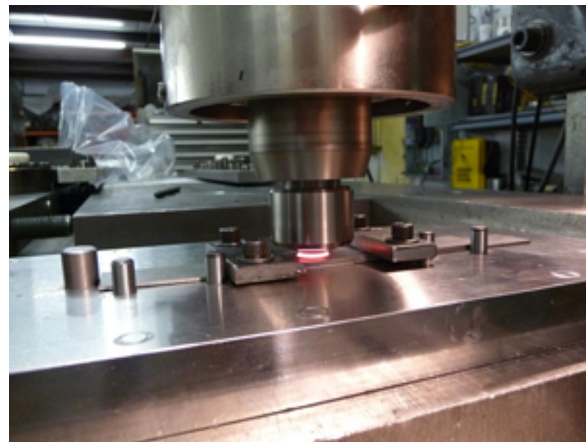
Figure 2. Plot of the variation in Z-loads throughout the life of PCBN variations Q60 and Q70 (left) and a visual of the FSSW process under load (right)
