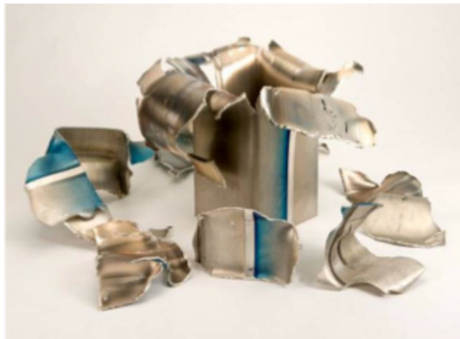
Figure 1. Mg extrusion exhibiting low ductility failure.
