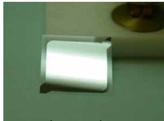
Individual glass layer with tabbed electrodes
