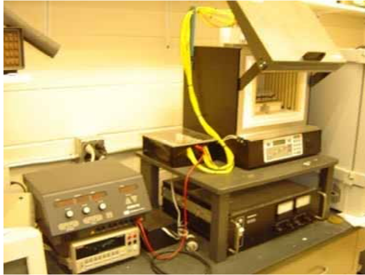
Fig. 4. Highly accelerated life test (HALT) system developed at Penn State University. Over 20 samples can be tested at time so that the failure mechanisms can be statistically determined.
