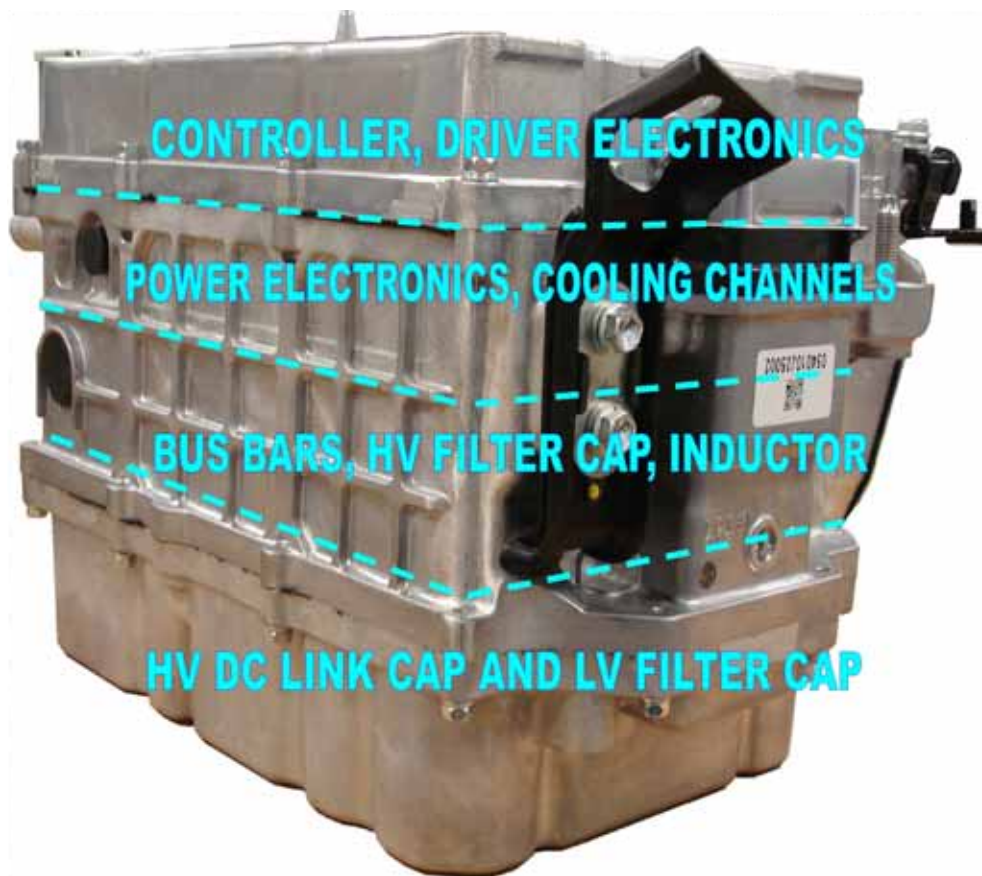
Fig. 1. The LS600h power converter unit.
