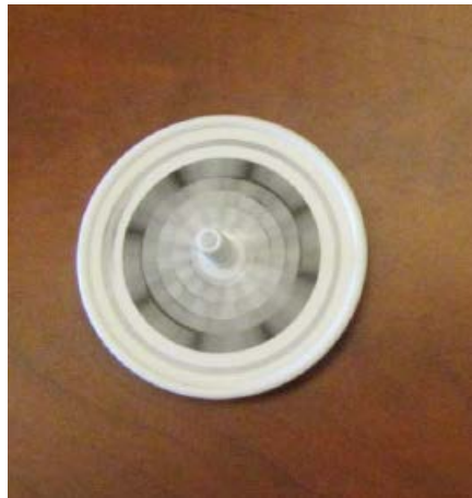
Figure 9. Flicker top showing “spokes” that indicate some flicker from an OLED luminaire and driver system dimmed with a 0-10V dimmer. (Photo: Leslie North)
