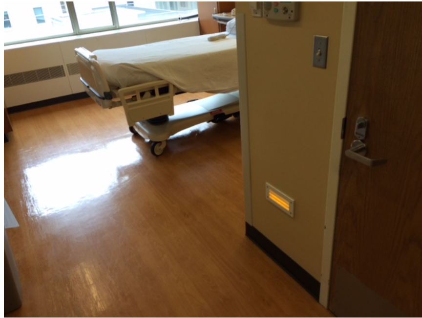
Figure A3: Hospital A patient room showing the step-light style wall-recessed amber nightlight near the door to the patient bathroom.
