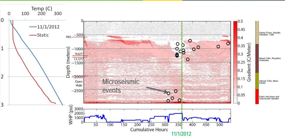
Although seismicity occurred above depth of 1500 m bgs, temperature profiles and gradients over 550 hour period indicate majority of fluid exited below 2500 m depth.
