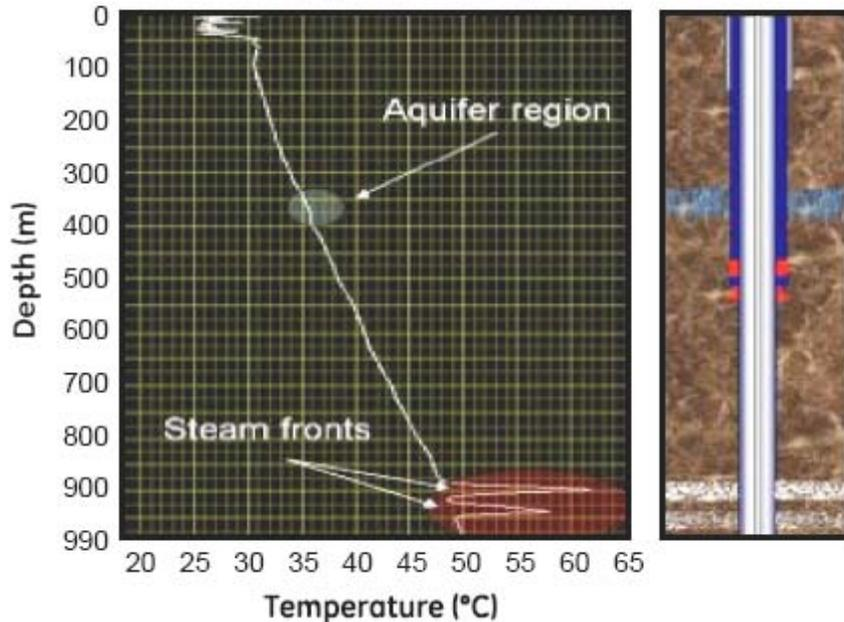
The effects of injection into the stimulation well are clearly seen when using DTS to monitor the recovery well to 1km deep
