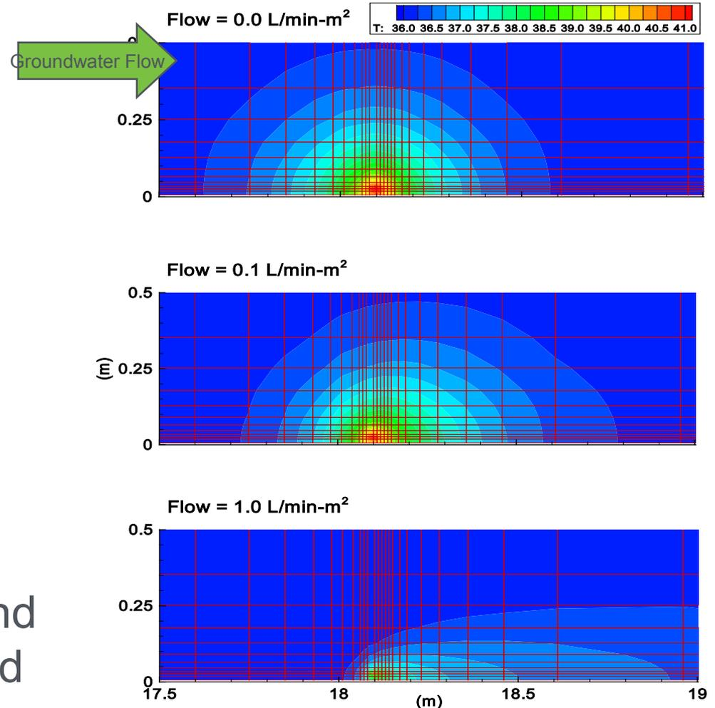
TOUGH2 Heat & Mass flow simulations of DTSPS system
