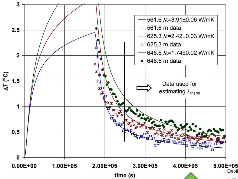
**Well logs for Ktzi201 and Ktzi202 showing temperature changes (dT) during DTPS heating and calculated thermal conductivities (TC) along with well layouts and lithologies [after Förster et al., GHGT-9, 2008].**
