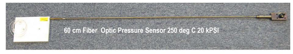
Successfully tested fiber Wellhead Outlet feed through at 250C and 20 KPSI
