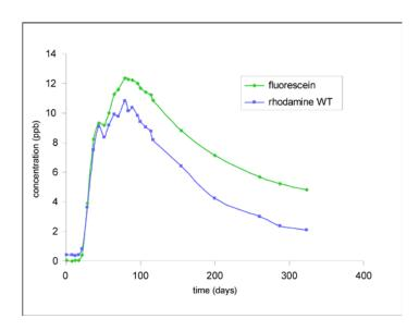
$$\frac{C_{1}}{C_{2}} = \frac{C_{1}^{o}}{C_{2}^{o}} \cdot e^{(k_{2}-k_{1})t}$$
