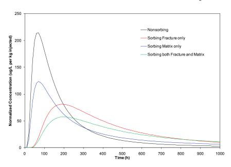
Breakthrough curve of a nonsorbing tracer and three possible breakthrough curves for a sorbing tracer depending on whether sorption is occurring only in fractures, matrix, or both.
