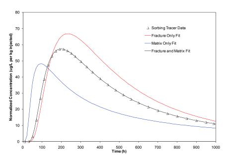
Assuming sorption only in fractures or matrix (red and blue curves) results in much poorer fits to the sorbing tracer breakthrough curve than assuming sorption occurs in both domains. The fracture surface area to volume ratio can be deduced from the best-fitting model parameters for the black curve.
