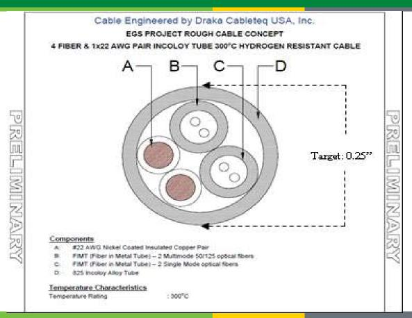
Complete Fiber/Copper Cable Solution for Long-Term Temperature and Pressure Measurement in Supercritical Reservoirs and EGS Wells
