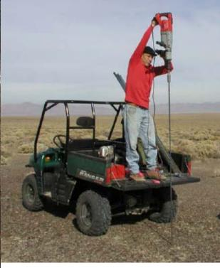
Black Warrior: Sub-soil gas and fluid inclusion exploration and slim well drilling
