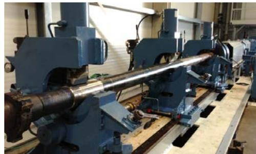
4<sup>3</sup>/<sub>4</sub>-in. metal-metal motor flow loop test
