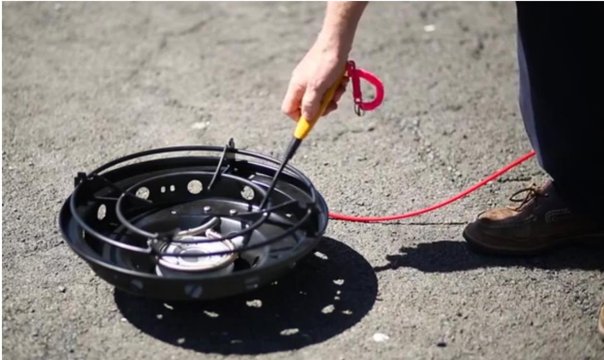
Figure 5. Small gas burner adapted for hydrogen and used to demonstrate hydrogen flame properties to training attendees.
