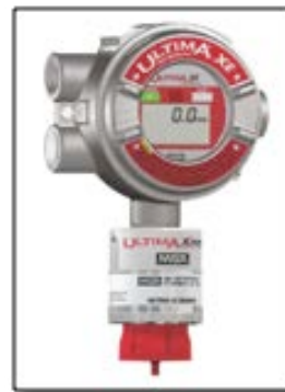
One safety feature of the generator is to have redundant hydrogen sensors, including the one shown here, which automatically shut down the generator and close all hydrogen tanks as soon as a hydrogen leak is detected.
