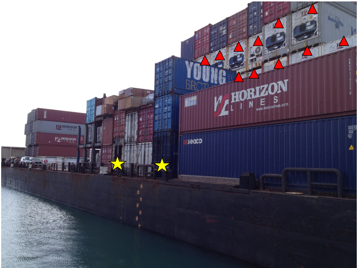
Figure 8: Loaded Young Brothers barge, showing location of diesel generators (yellow stars) and reefers (red triangles).
