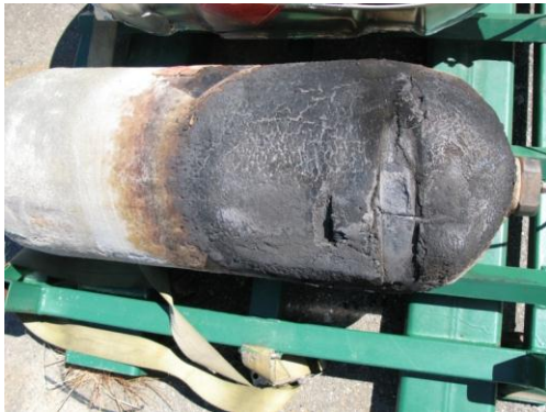
Intumescent epoxy after 30 min @ 1000 deg C test
