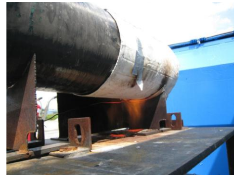
Thermal wrap undergoing localized fire
