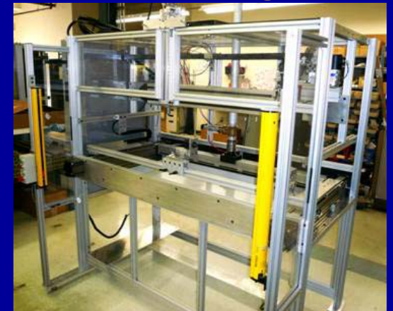
Automated Cathode Coating
