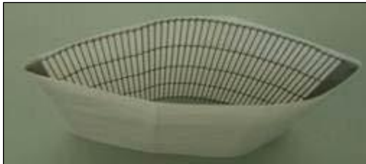
Figure 198. Plate Frame Membrane Humidifier single cell pouch (Source: Johnson, William B. "Materials and Modules for Low-Cost, High-Performance Fuel Cell Humidifiers," W.L. Gore & Associates, Inc., presentation at the 2012 DOE Hydrogen and Fuel Cell Program Annual Merit Review, Washington, DC, 17 May 2012.)
