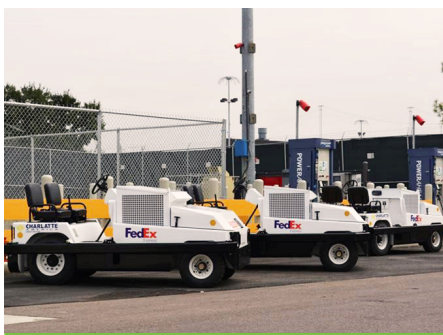
Fuel cell ground support equipment at the FedEx Express hub at the Memphis Airport
