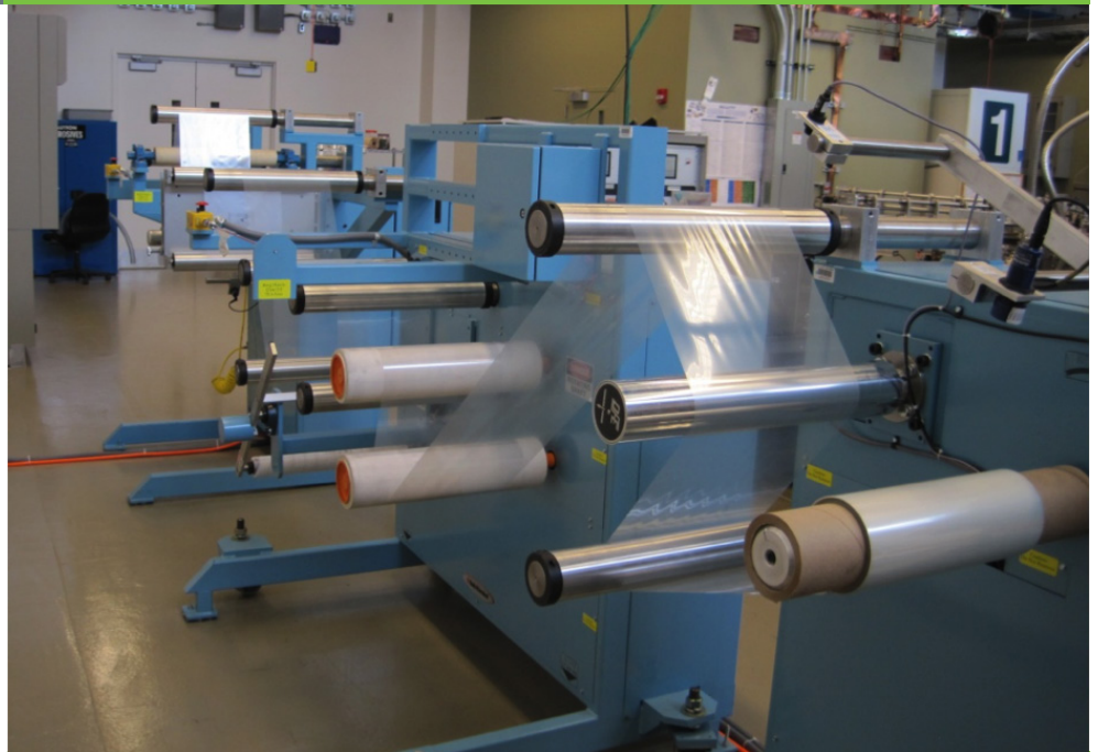
Figure 1. Industrial-style roll-to-roll web-line at the National Renewable Energy Laboratory. The web-line is used to develop and validate in-line inspection methods for fuel cell components, including membranes, electrodes, and gas diffusion media.
