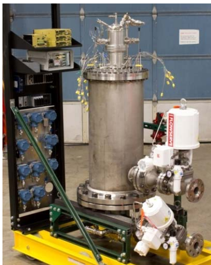
PCI 250kW Autothermal Reformer
