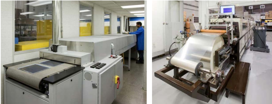
Figure 3. (Left) screen printing and (right) tape casting. Photos from M. Richards, Versa Power Systems
