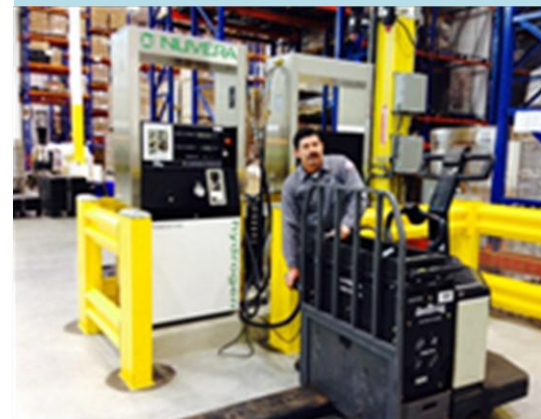
Golden State Foods forklift operator fueling a material handling vehicle with hydrogen, using a Nuvera PowerTap refueling system.
