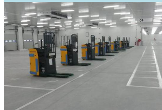
Forklifts equipped with Plug Power fuel cells at Prelogis' warehouse in France
