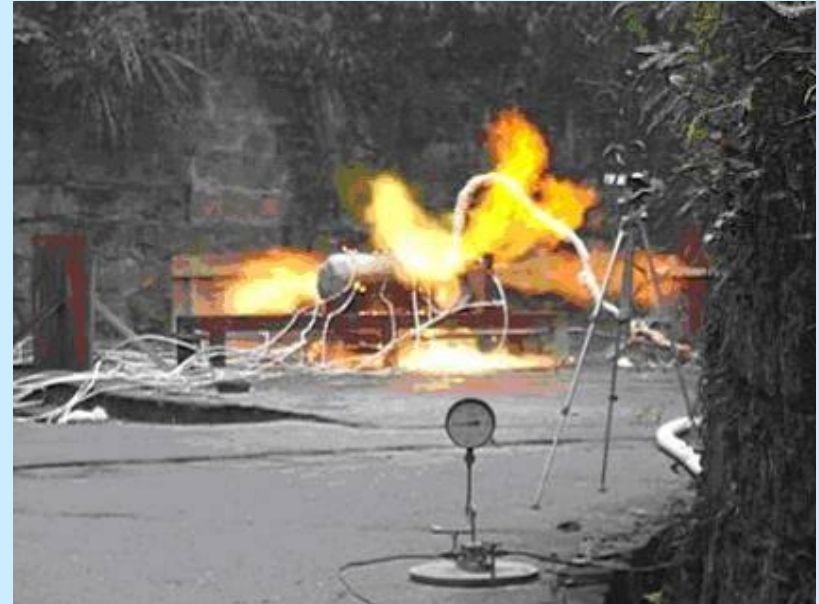
Hydrogen deflagration after PRD was activated
