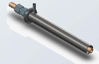
3 kWth Diesel SR w. endo & exothermic sections
