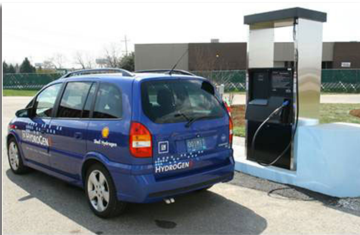
H2 ProGen Hydrogen Dispensing Station
