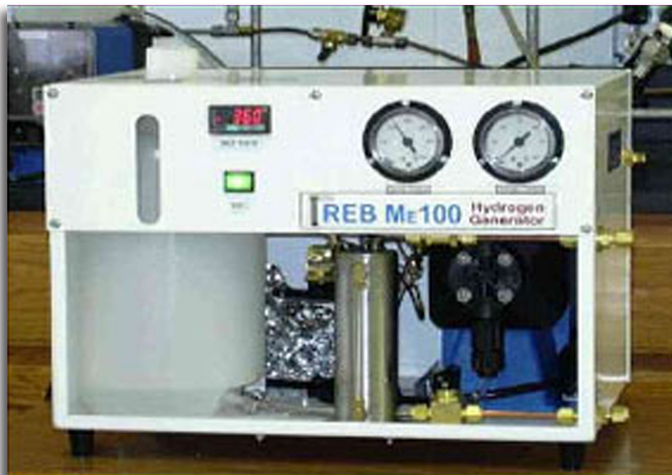
The ME100 Generator System
