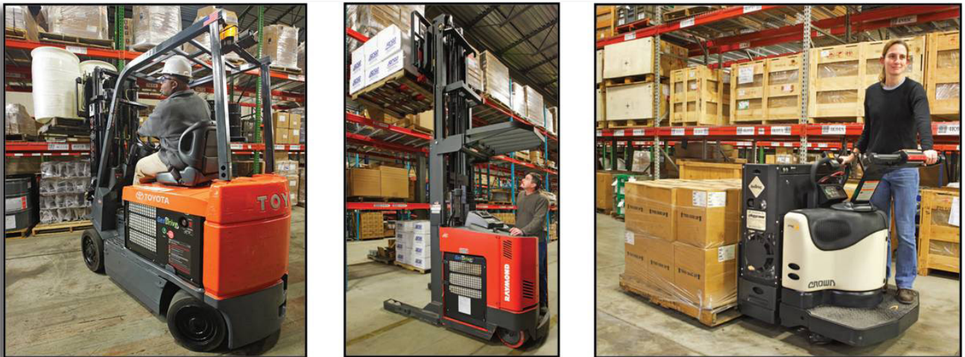
Class-1, -2, and -3 Forklifts (shown from left to right) Powered by Plug Power's GenDrive Fuel Cells
