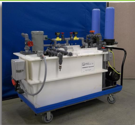
FARADAYIC® ElectroCell Technology For Manufacturing PEM Bipolar Plates using The FARADAYIC® ElectroEtching Process
