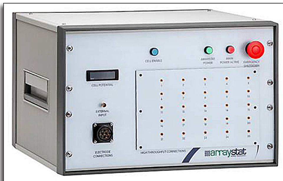
NuVant's Automated 25-Channel Array Potentiostat (Arraystat)
