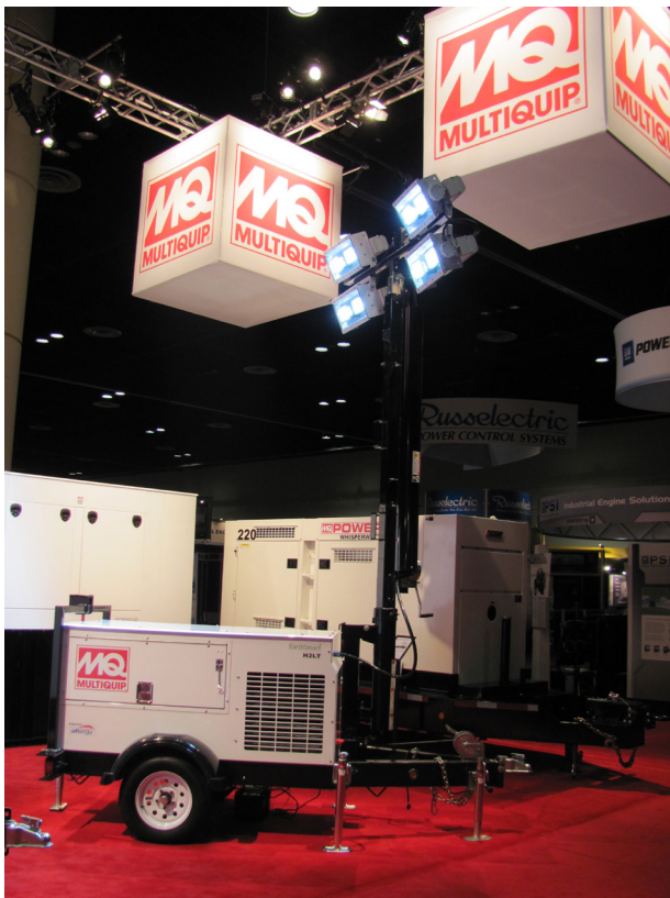
Sandia's Fuel Cell Based Mobile Lighting System by Multiquip Inc.
