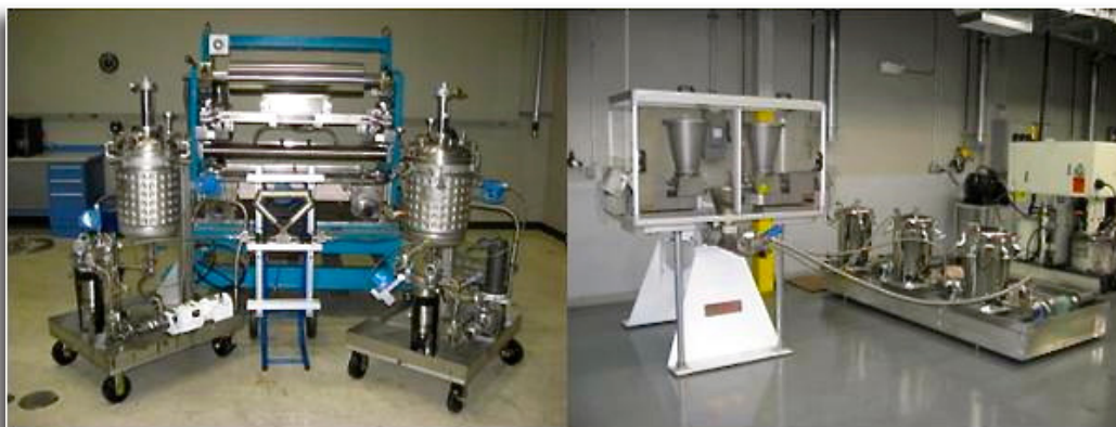
AvCarb's Continuous Mixing and Multilayer Coating Equipment
