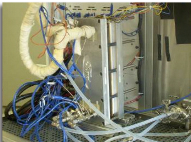
Fuel-Cell Stack Using TreadStone's Bi-polar Plates on the Testing Station at Ford Motor Company
