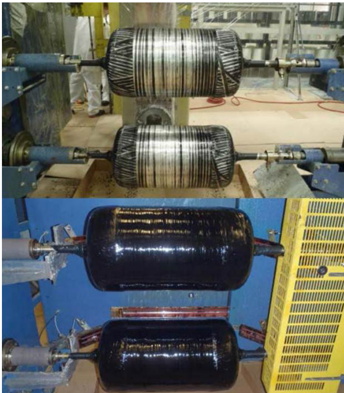
Glassfiber Layer Wound with CNT Epoxy (Top) and After Epoxy Resin is Smoothed (Bottom)
