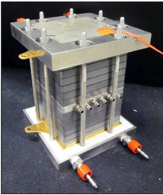
RPI's Test Fuel Cell Stack Using 50 cm 2 MEAs
