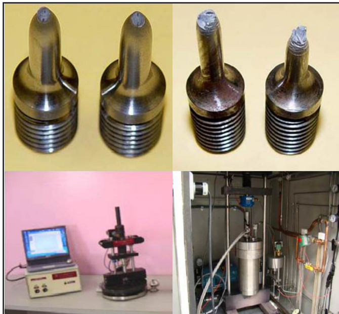
Test Sample Failures (LHS Cup & Cone RHS Faceted Surface) and High Pressure Test Equipment
