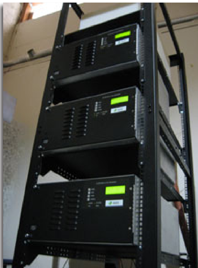
Genesis Fueltech's Model 20L Reformers
