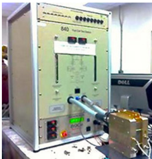
USC's MEAs in a Prototype Test Fuel Cell Stack (top) Durability & Performance Evaluation Testing Equipment (bottom)
