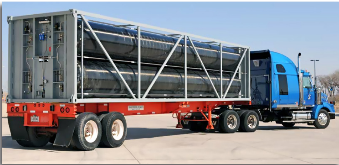
Hexagon Lincoln's 3,600 psi TITAN™ Tank and Frame System
