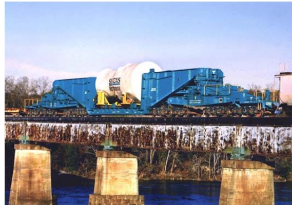
Fig. 2.4.7 Schnabel car - a twenty-two axle rail car, built in 1969, originally owned by Westinghouse. This car, used to deliver generators, is now owned by Siemens-Westinghouse, Ontario, CAN.
