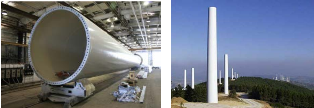
Fig. 1.1.1 Tower Section after Paint and Installed Towers
