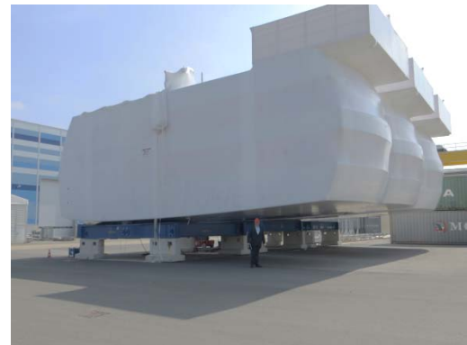
Fig. 2.10.4 REpower 5MW nacelle ready for deployment from the Bremerhaven GmbH port.
