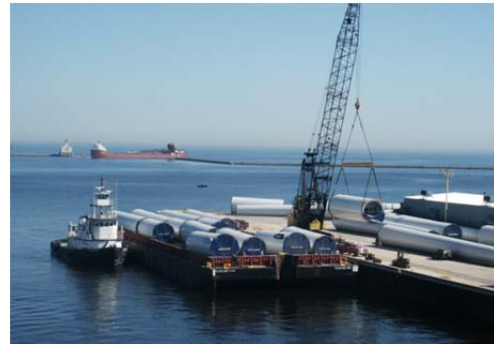
Fig. 2.2.7 Tower Transport by Barge
