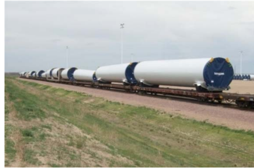
Fig. 2.2.5 Tower Transport by Rail
