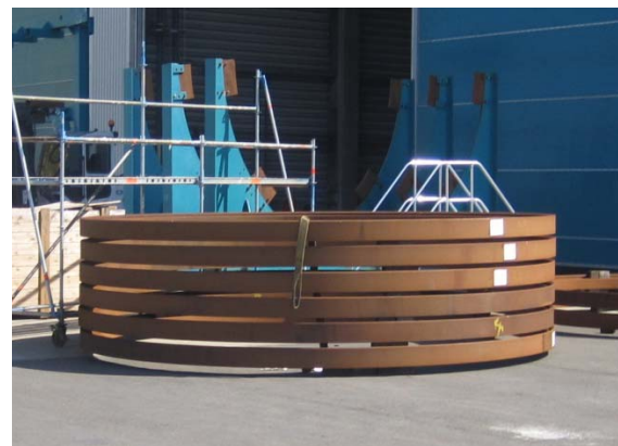
Fig. 2.11.2 Forged tower flanges ready for cleaning and tower assembly in Germany.
