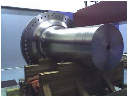
Fig. 2.12.2 Machine shaft 45,000 lb., 15' long and 8' diameter. McSwain Manufacturing, Ohio.
