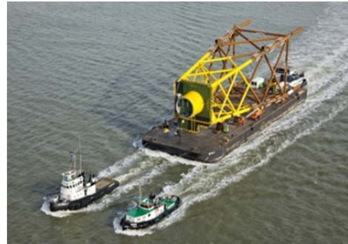
Fig. 2.5.6 - Muller Dordrecht horizontal transport of a 900 ton jacket foundation near Belgium.
