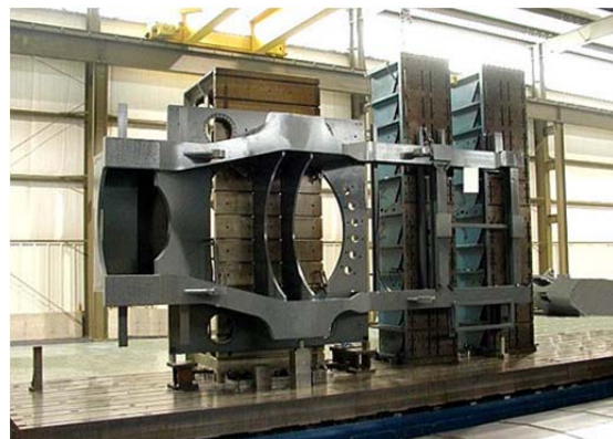
Fig. 2.8.2 K&M Machine Fabricators main frame in production
