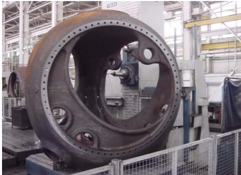
Fig. 2.7.1 Cast 1.5MW cast hub, ready to be machined. Location: HPM in OH.
