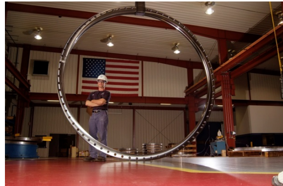
Fig. 2.11.1 Forged and machined yaw ring for a 1.5MW application. A product of Rotek, Aurora, Ohio
