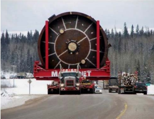
Fig. 2.4.6 Truck transport of Exxon Mobile refining equipment for Canadian Tar Sands project. Load width is 24ft – compare to the 5MW generator at 21.3 ft.
