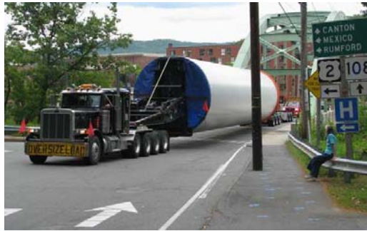
Fig. 2.2.6 Tower Transport by Truck
