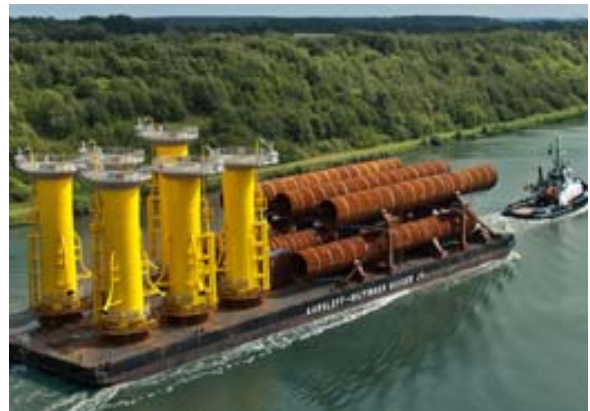
Fig. 2.6.7 Barge transport by Bilfinger Construction – London Array
