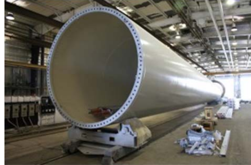
Fig. 2.2.1 Trinity Tower Section
