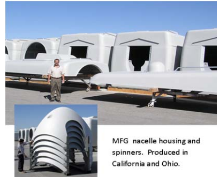
Fig. 2.10.1 Nacelle housings and spinner covers produced by MFG and Wausaukee Composites
