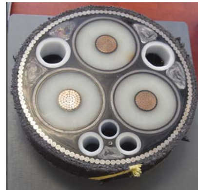
Fig. 2.13.1 Subsea cable cross section, 19” diameter cable. Wolf Island Wind Project Canadian Renewable Energy Corp.
