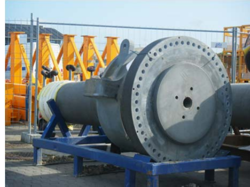
Fig. 2.12.1 Main shaft with flange for a 1MW. Forging is 28 in x 74 in x 7 ft. at the head
