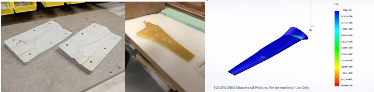
Figure 9: Negative molds for the blades (left), foam blade made from molds (middle), finite element analysis for blade design using selected foam at 2500 RPM.
