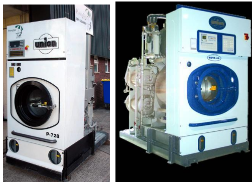
Figure 8-30: Traditional PCE Dry Cleaning Machines
