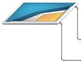
Figure 6-35: Flat-Plate Collector for Solar Thermal Water Heating System
