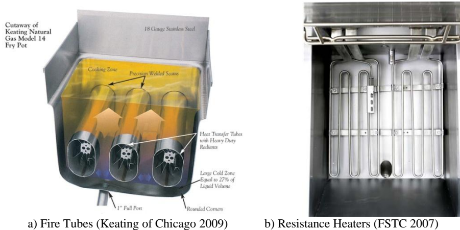
Figure 2-3: Fire Tubes in a Gas-Fired Fryer and Electric Resistance Heaters in an Electric Fryer
