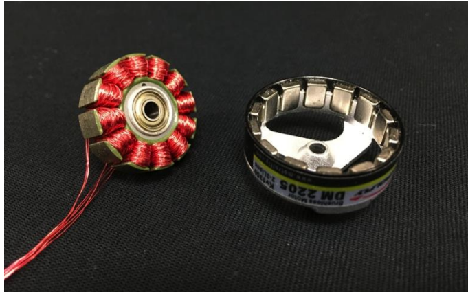
Fig. 3.14: Motrolfly motor assembly
