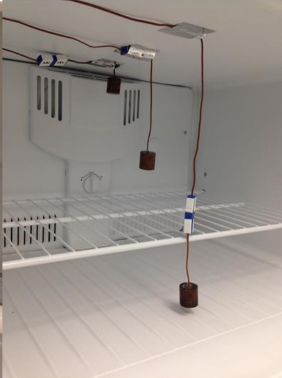
Fig. 2.11: Pictures of thermocouples in fresh food (left) and freezer (right) compartments
