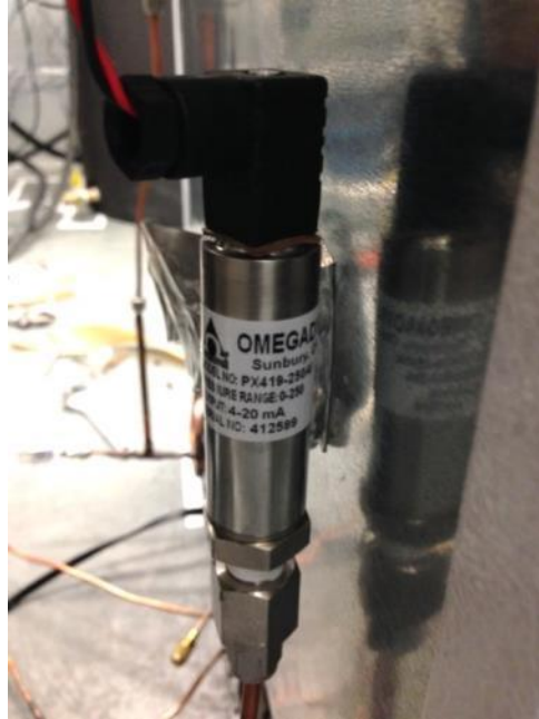
Fig. 2.13: Pressure transducers used in the test
