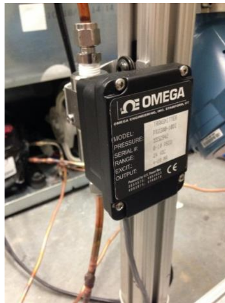
Fig. 2.14: Differential pressure transducer used to measure the condenser pressure drop.
