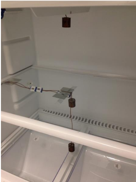
Fig. 2.11: Pictures of thermocouples in fresh food (left) and freezer (right) compartments
