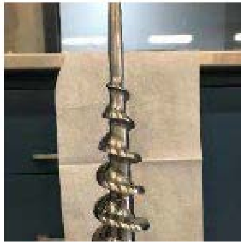
Wear on SS316 auger from corn stover (light wear – left & significant wear – right) FCIC peer review image
