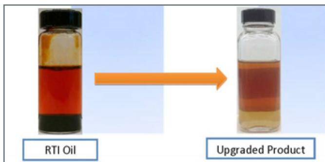
The goal of the project is to demonstrate an advanced biofuels technology that integrates a catalytic biomass pyrolysis step and a hydroprocessing step to produce infrastructure-compatible biofuels. Research Triangle Institute (RTI) International is developing a novel single-step catalytic biomass pyrolysis process to produce a hydrocarbon-rich, bio-crude intermediate. Our partner,
