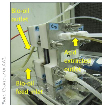
Problems with stability due to the presence of organic acids have created major technology hurdles for bio-oil that cause problems in storage and transportation. Removing carboxylic acids will reduce acidity and oxygen of the bio-
