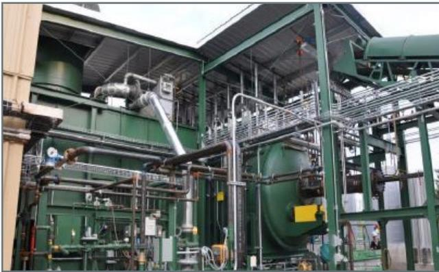
The objective of this DOE integrated biorefinery project has been to build, test, optimize, and validate a 25 dry-ash-free, ton (daft)-per-day plant for the conversion of
