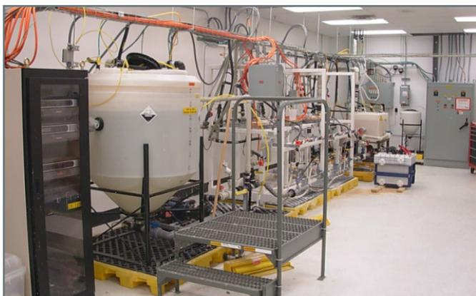
The University of Nevada, Las Vegas and an industrial partner, Ceramtec, are developing a tubular Sodium Super Ionic Conductors (NaSICON) membrane-based process that produces high-purity sodium methoxide from low-cost aqueous sodium hydroxide. An electric
