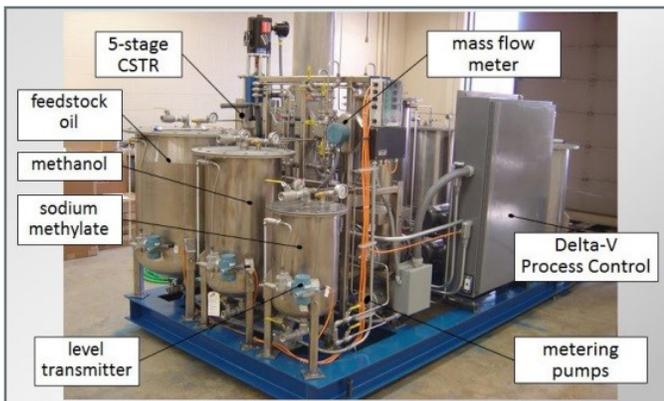
The purpose of this research is to demonstrate the feasibility and economic viability of a biodiesel micro-refinery and a micro-scale biomass gasification facility. A fully integrated, demonstration-scale biodiesel micro-refinery is being built upon a recently developed core subsystem. The biomass gasification unit is
