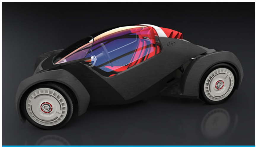
Local Motors collaborated with large-scale manufacturing system builder Cincinnati Incorporated, advanced materials research pioneer, Oak Ridge National Laboratory (ORNL), and SABIC to develop and validate the technology and materials needed to deliver the world's first 3D-printed vehicle, the Strati, at IMTS 2014. (Photo courtesy of SABIC)
