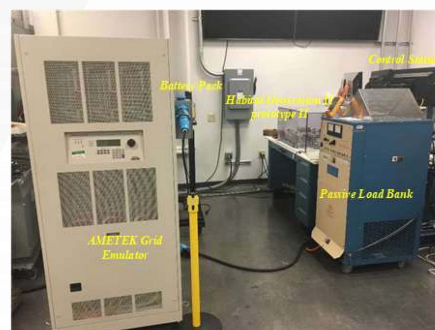
Test Setup for Grid Tied Operation
